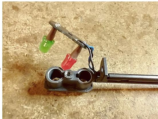
🇬🇧 6. Insert the two LEDs into the slots where the light bulbs were previously placed: the green LED goes at the top, the red LED goes at the bottom.
