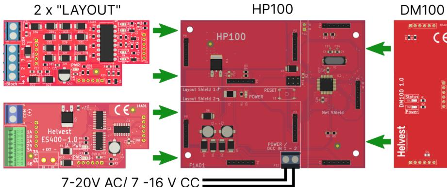
To operate the decoder as described, neither a digital control unit nor a computer is required. Connect the HP100, DM100, and the two 'Layout' modules as shown in the figure. The HP100
