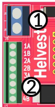
**3 - The outputs A and B of each device (1A and 1B, 2A and 2B etc.) are powered only when the device is selected by the control unit.**
